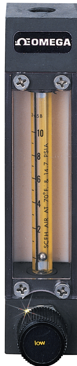
FL-1705-V, $172, rotameter with optional 316 SS control valve, shown actual size.
