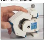
Step 2: Loop Tubing Over Rollers. No Need to Thread!
