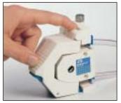
Step 4: Tighten Screw to Secure Tubing
