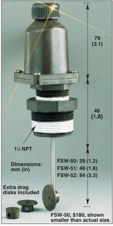
FSW-50 Series: Polyphenylene sulfide, 316 SS, FKM; also available with polyphenylene sulfide, Hastelloy C and FKM construction Electrical Cable Fitting: Water resistant for cable diameters 0.250 ±0.025" Weight:
