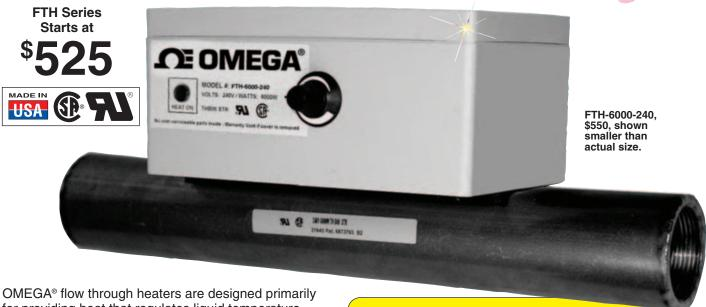
OMEGA® flow through heaters are designed primarily for providing heat that regulates liquid temperature from 32 to 88°C (90 to 190°F). The heaters have a titanium element that resists corrosion. The flow through tube is 381 mm (15") long and has 1 NPT female pipe connections and is available in 304 SS. The safety high limit trip point for the heater is 99°C (210°F). The 201 x 145 x 89 mm (7.9 x 5.7 x 3.5") enclosure is made of ABS plastic and is water resistant.
