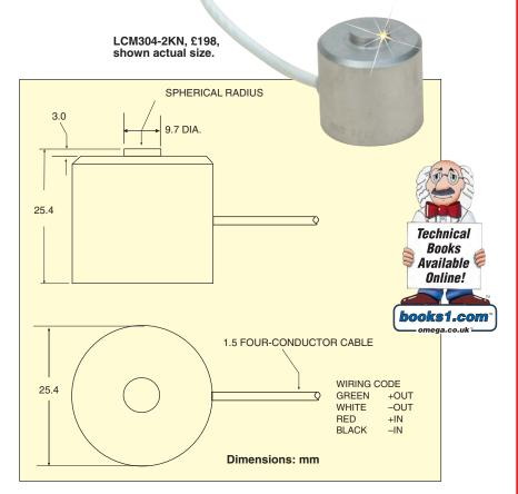
Safe Overload: 150% of capacity Ultimate Overload: 300% of capacity Bridge Resistance: 360 Ω minimum
