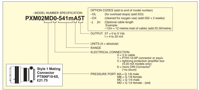
Ordering Examples: 1.) PXM02MD1-541mAl-MB is a 541 to 1080 mbar calibrated electronic barometer with G 1/4 internal thread, 4-20mA output, a Bendix connector and the optional mounting bracket, £570 + 28.50 = £598.50. Mating Connector: (not included) PT06F10-6S, £21.75.
