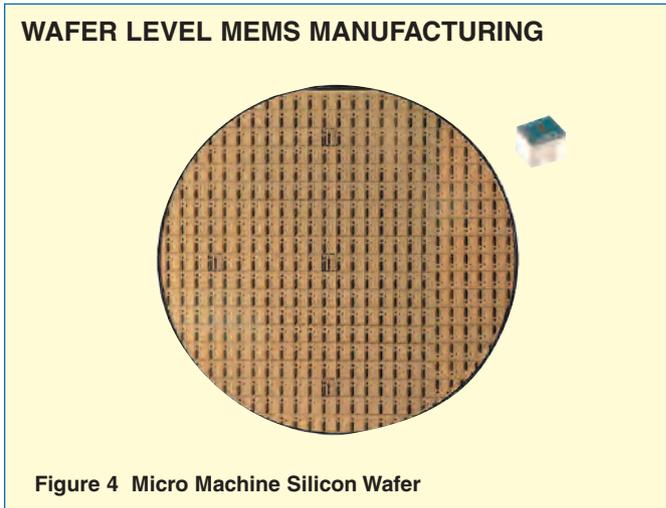
MicroElectroMechanical systems (MEMS) are the twenty first century solution to these drawbacks. MEMS are mechanical silicon structures that can be fabricated at the wafer level (Figure 4). **Characteristics such as high sensitivity, small size, low signal to noise, excellent repeatability and low hysteresis, high overload, high yields, process repeatability have made Micro Machine Silicon the sensing element of choice for building reliable, flexible and stable pressure sensing devices.**
