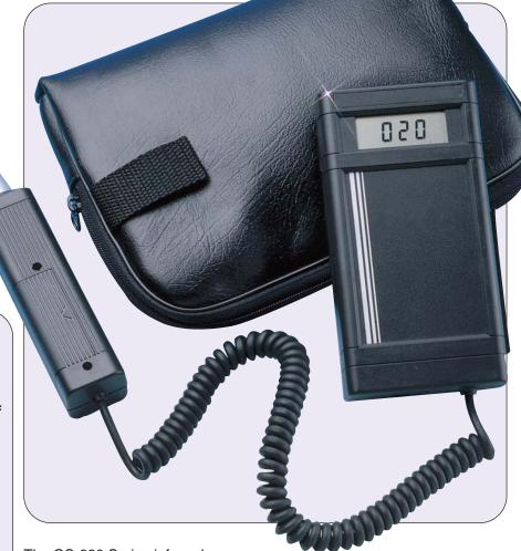
The OS-620 Series infrared energy meters have the additional feature of measuring heat loss (or gain) through walls and windows without physical contact. These versatile units are designed to measure the temperature of building materials such as paper, plaster, ceramic, stone, concrete and glass that have emissivities between 0.9 and 1.0.
