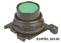
The E34 Series 30.5 mm pushbutton line features the same rugged die cast construction of our 10250T line with an additional two layer 100% solid thermosetting cathodic epoxy coating. This coating provides a flat black smooth, consistent, corrosion resistant surface that has passed a demanding 600 hour salt spray test. (The industry standard for this 4X test requires only 200 hours). E34 cathodic coating is not recommended for use in applications where
