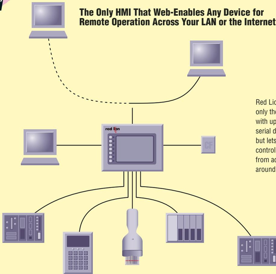
Red Lion's G3 HMI Series is not only the first to communicate with up to five different types of serial devices simultaneously, but lets you access, monitor and control these devices remotely—from across your network, or around the globe.
