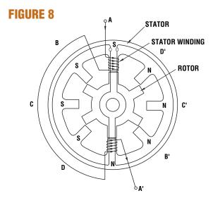
4 phase VR motor with one phase on.
