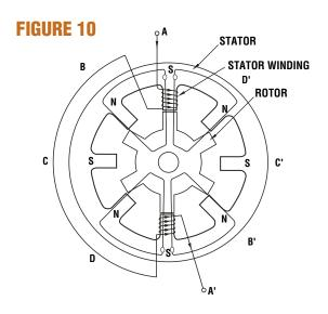
4 phase VR motor with one phase on. Wound for alternate polarity.
