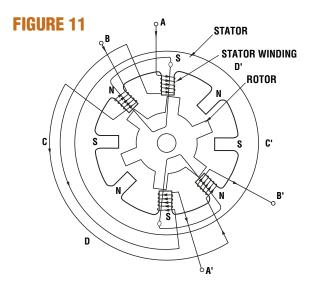
4 phase VR motor with two phases on. Wound for alternate polarity.
