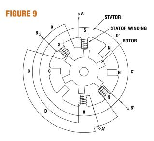
4 phase VR motor with two phases on.
