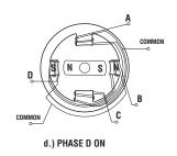
PM step motor with half step motion.
