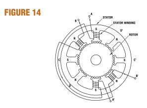
Diagram of 1.8 $^{\circ}$  VR motor.
