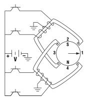
Schematic diagram of a PM motor.
