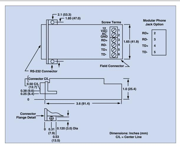
A self-powered model and a host-powered model are available. The self-powered unit uses 12 Vac from a wall-mounted transformer while the host-powered unit takes ±DC power from pins 9 and 10 of the RS-232 connector. The modem circuits—and, consequently, the host device—are protected from electrical transients due to lightning strikes or operation of heavy industrial equipment.
