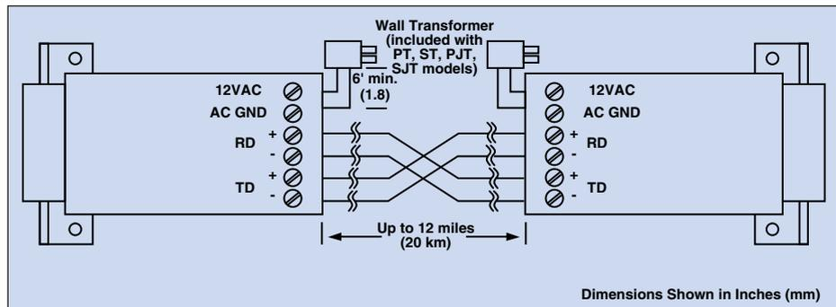
The LDM70 Series of products is designed to allow video display terminals (VDTs) and other RS-232 devices to be connected over distances sufficient to cover any industrial or institutional complex of buildings. These modems feature a rugged aluminum enclosure small enough to mount on the back panel of VDT units, saving valuable desk and floor space.
