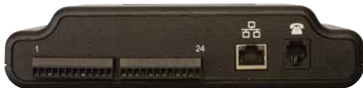
Bottom view of OMA-VM606E showing ports.
