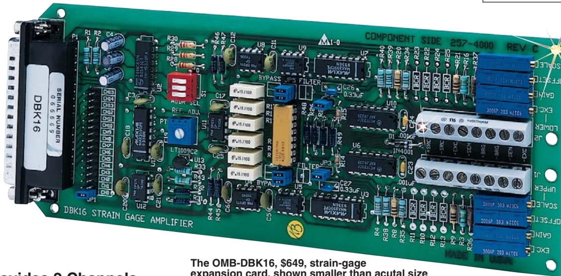
The OMB-DBK16, \$649, strain-gage expansion card, shown smaller than actual size
