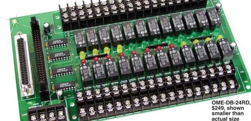
Power Consumption: +12 V @ 528 mA max; +5 V @ 150 mA max
