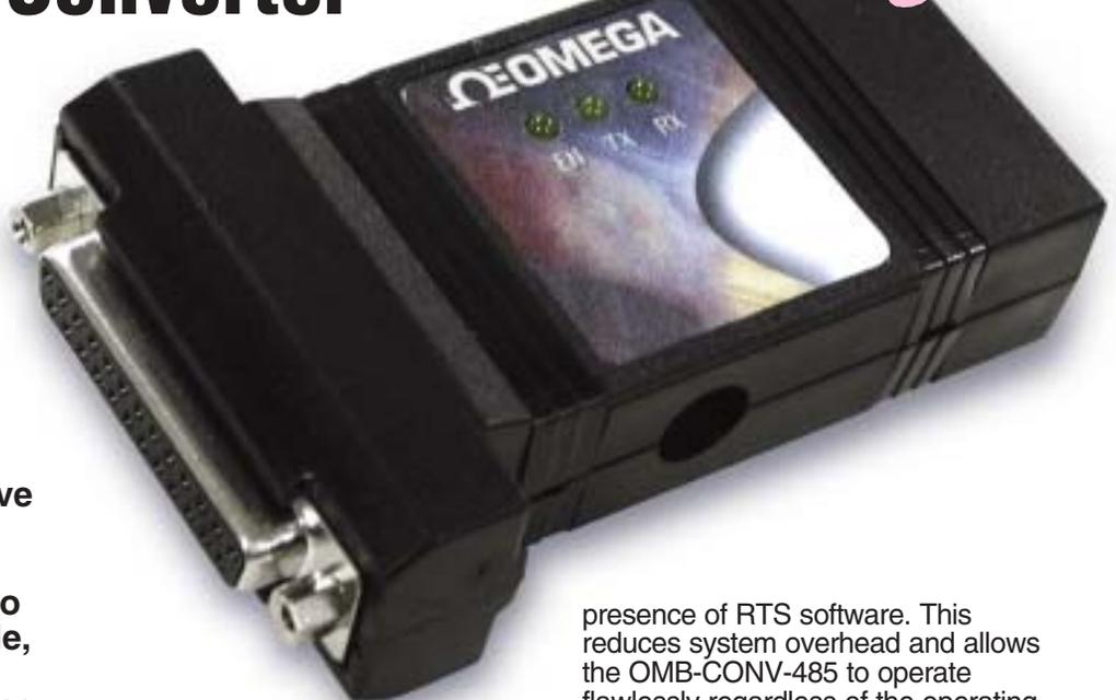
The OMB-CONV-485-ISO is an isolated version of the OMB-CONV-485. Isolation is important in installations where the equipment connected to the PC is either located far from the host system, or on a different power transformer circuit. Isolation on the OMB-CONV-485-ISO eliminates the effects of ground loop current, a commonly neglected and misunderstood phenomenon that leads to data errors and the destruction of communications equipment.
