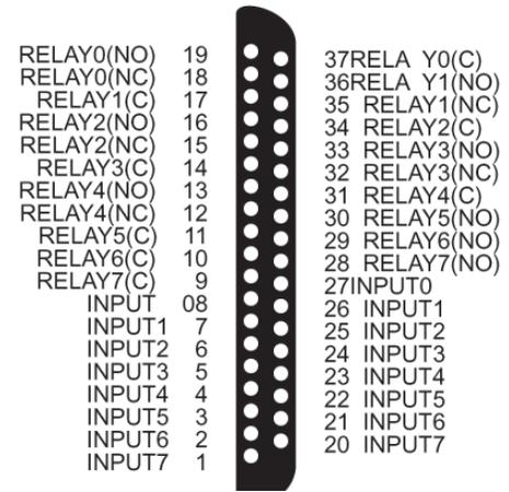
**PCI-PDISO8 37-Pin Connector**
