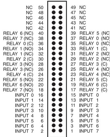
**PCI-PDISO16 50-Pin Connector**
