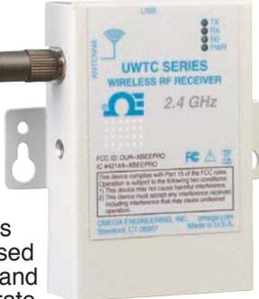
With the UWTC-REC1 data from up to 48 wireless connectors or probe assemblies can be received and displayed on your PC simultaneously. This receiver connects to an unused USB port on your computer and must stay connected to operate and receive data.
