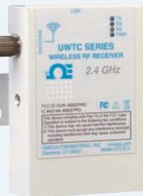
UWTC-REC2 wireless receiver with analogue output, see receivers on page S-9 and S-10.
