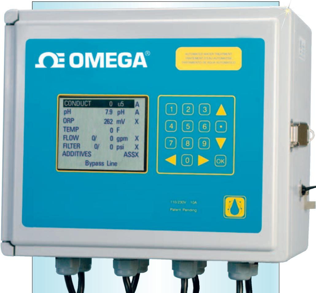
The CDCN13 has 8 control relay outputs, for up to 4 chemical additives, fill valve, bleed valve, probe rinse, and remote alarm. Standard features also include dynamic probe failure testing for pH/ORP sensors, allowing the controller to detect a probe failure quickly after it occurs, so the user can avoid dangerous out-of-range conditions. The automatic probe rinse can be used for either manual or automatic cleaning of pH or ORP electrodes.
