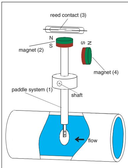
The reed contact used as a sensing element consists of two ferro-magnetic contact blades located in a glass bulb filled with inert gas. This practically eliminates wear resulting from contact burning. This construction allows a useful life of up to 100,000,000 switching cycles.
