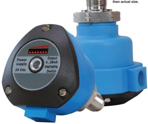
connection of the FSW-9000 Series are made with 316 SS and the standard enclosure is glass-filled nylon. The FSW-9000 Series can be made with a great variety of process connections such as threaded, flange, or sanitary and is also available in an aluminum enclosure for hazardous environments. Intrinsic safety barriers required for explosion proof areas.
