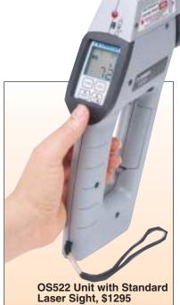
With a combination of powerful features, the new portable and rugged OS520 Series infrared pyrometers offer solutions for many non-contact temperature measurement applications. The standard 1 mV per degree analog output allows interfacing with data acquisition equipment, including chart recorders, dataloggers and computers.
