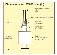
Switch Actuation: Approximately ½ the distance from the end of stem to mounting or halfway point of float travel Lead Wires: 20 AWG. 24" PVC
