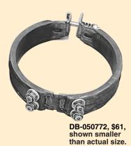
Ten times the life-only slightly higher cost. This economical long life heavy duty band heater has a %" thick chrome steel (stainless) sheath, which offers ten times the life of a mica band heater at only a slightly higher cost than mica, and considerably lower than ceramic band and aluminum shoe designs.
