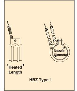
Thermocouple holes, plugs ,and extended leadwire and braid are available. See page H-14.
