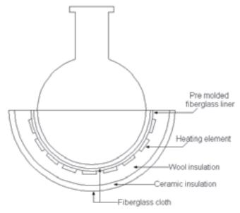
Cutaway view of lower Hemispherical Heating Mantle.
