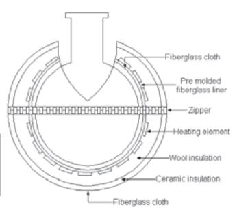
**Cutaway view of Spherical Heating Mantle.**
