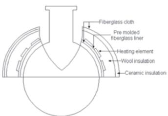
Cutaway view of Upper Hemispherical Heating Mantle.
