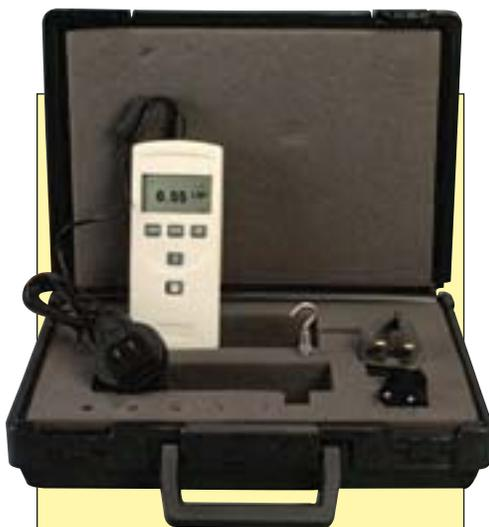
Comes complete with hard carrying case, two 9 Vdc batteries, universal battery eliminator, hook, flat tip, calibration certificate, and operator's manual.
