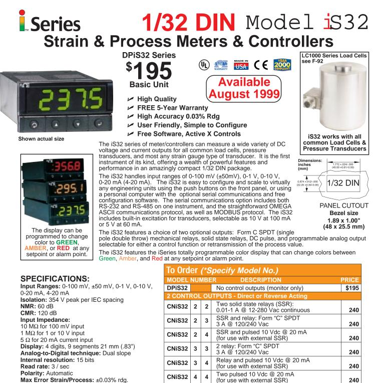
Span tempco.: ± 50 ppm / C Step response: 1-2 sec. Warmup to rated accuracy: 30 min. Analog Output (optional): 0-10 V, 4-20 mA, can be used as Retransmission or PID Control. Excitation Voltage: 10 V @ 100 mA, 5 V @ 60 mA Power: 90-240 Vac 50-400 Hz or 90-375 Vdc, 4 W or (optional) 24 Vac 50-400 Hz or 12-36 Vdc. 5 W Dimensions: 48 H x 96 W x 127 D mm (1.89 x 3.78 x 5.0") Weight: 295 g (0.65 lb) Approvals: CE per EN50081-1, EN50082-2, EN61010-1
