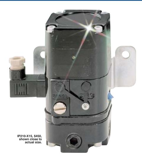
The IP210 provides a reliable, repeatable, accurate means of converting an electrical signal into pneumatic pressure. Its force balance principle is a coil suspended in a magnetic field on a flexible mount. At the lower end of the coil is a flapper valve that operates against a precision ground nozzle to create a backpressure on the servo diaphragm of a booster relay.
