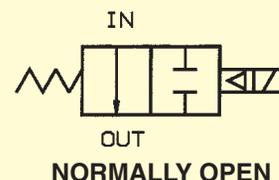
Port Identification: Flow arrow on body indicates flow direction—ports are not marked.
