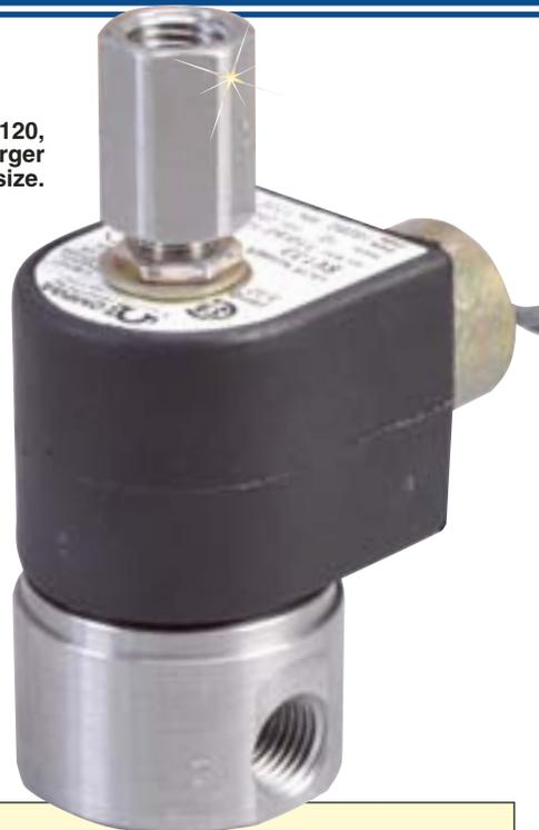
through the valve. When current flows through the coil, a magnetic field is produced and it turns the stop into an electromagnet that attracts the magnetic plunger.
