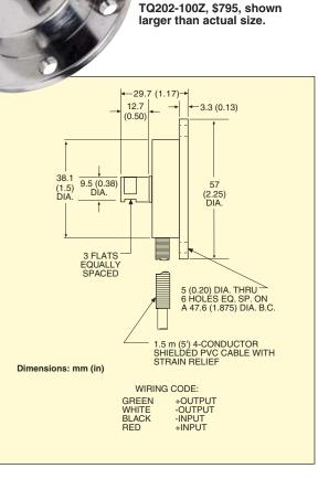
Safe Overload: 150% of capacity Ultimate Overload: 300% of capacity Construction: Stainless steel Electrical: 1.5 m (5') 4-conductor shielded PVC cable with strain relief Protection Class: IP65
