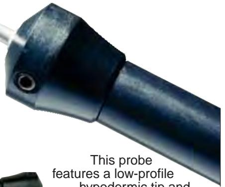
This probe features a low-profile hypodermic tip and convenient handle for short depth penetration of soft materials such as rubber. A grounded junction, 300 mm (1') of retractable cable (which stretches to 1.5 m [5']) and a subminiature male connector are standard. The handle is rated to 162°C (325°F).
