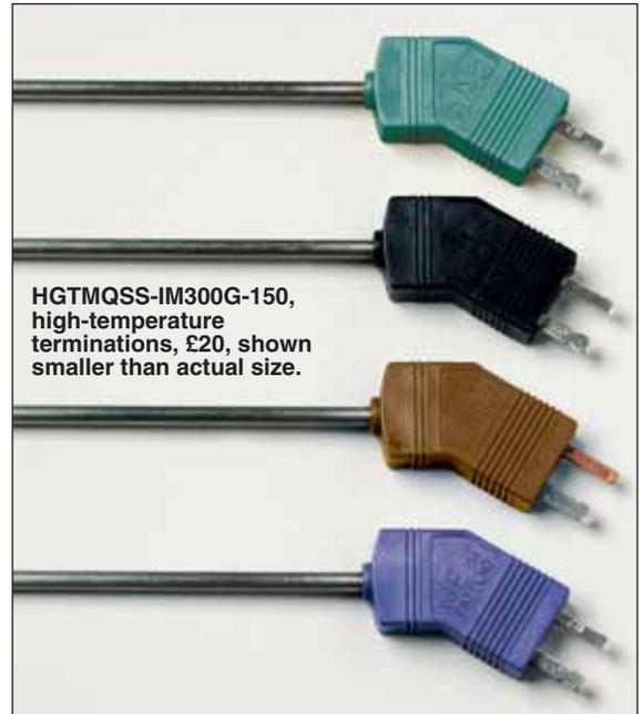
The OMEGA® low-noise thermocouple probes and connectors maintain an electrical connection from the sheath of the probe, through the connectors, all the way to the user's instrumentation. This system ensures highly accurate measurements by protecting against electrical noise. The external strap maintains the electrical connection of the ground wire and strengthens the link between the 2 connectors. The female connector features a handy write-on area, for easy identification.
