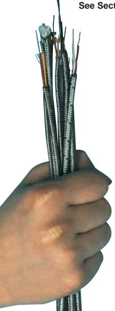
OMEGA can overbraid any thermocouple wire with either Inconel 600, 304 SS or Tinned Copper overbraiding. Both Inconel and Stainless Steel overbraiding add durability, flexibility, and abrasion protection to your valuable thermocouples, thus lengthening the life of your thermocouple by protecting it from wear. Low cost Tinned Copper overbraiding provides electrical shielding with the added benefits of durability, flexibility, and abrasion protection.
