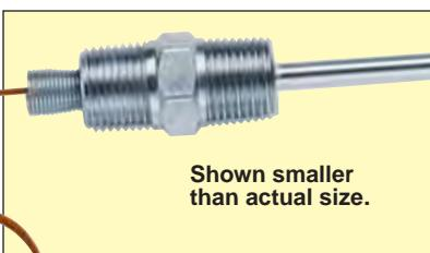
This flexible lead-wire replacement probe is ideal for field installation with existing protection heads or for extending leads to remote locations. Flexible leads prevent breakage in hard-to-wire situations. These probes have 20 AWG stranded lead wire and a 1/8 x 1/2 NPT hex fitting. Probe length includes 13 mm (1/2") of hex fitting threads.
