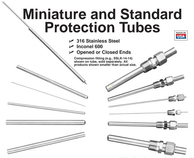
OMEGA® miniature and standard protection tubes are available in 316 stainless steel and Inconel 600 nickel alloy. Tubes are available either opened at both ends or with one end closed. Standard length available from stock is 150 mm (6"); however, practically any length tube is available on short delivery.
