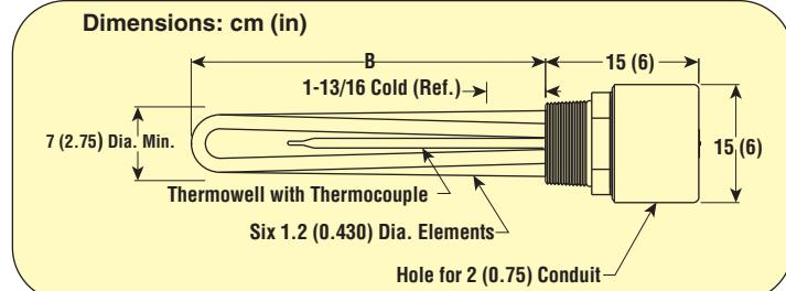
OMEGALUX® field adjustable screw plug immersion heaters can be applied to a variety of clean water and oil applications. The unique versatility of this design allows field adjustment of the rating by simple connections to the six elements of
